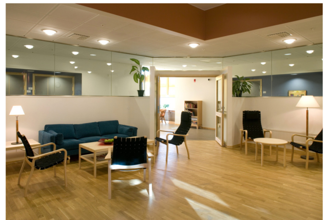
Fig. 3. Portion of a communal central area of a ward in New hospital showing groupings of movable and semi-movable seating. Half-wall partitions of break resistant glass enable staff moving in the central area to observe bedroom doors.
